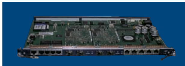
6022: Mobile WiMAX IDU serving 2 sectors MIMO A/B Matrix
